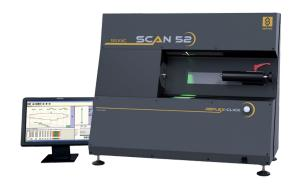
As the measurement is being taken, the part is maintained on the carriage while the area around the data point is illuminated with a green parallel light. A part image is then projected on the highresolution CCD linear sensors, acting as light detectors. All emitted signals are then analysed and computed as measured values.
